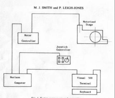
Fig. 1. System components and connections
